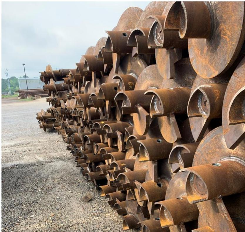
Pictured above, the toe of the pile is plugged by welding a steel plate to the ID of the pipe. The grout port, through which grout is delivered under pressure to fill the void created as the driver plate advances through the soil, can also be seen
