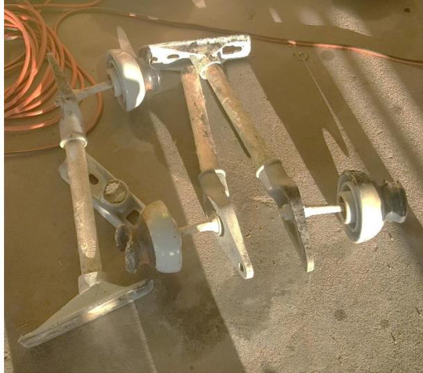
Figure 4 – Surface Corrosion on the End Fittings
