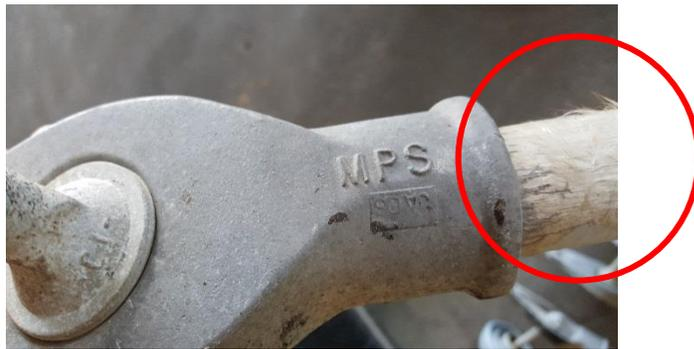
Figure 1 – Blooming of the Fiberglass Rod Surface
