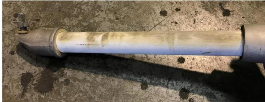
Figure 2 – Contamination Buildup Along the Fiberglass Rod Surface
